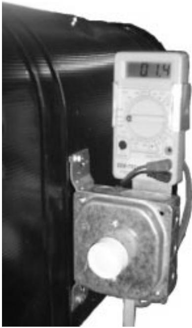
For the annealer, I mounted a steel electrical box on the mailbox, and used a steel switch face plate. The box and face plate act as a heat sink. The face plate stays cool enough for a glass worker to keep a hand on - probably below 115°F.
