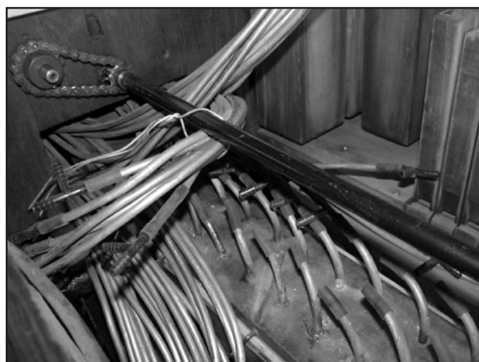
Figure 7. A closer view of the tubing closest to the key frame on the left of the Bruder.
