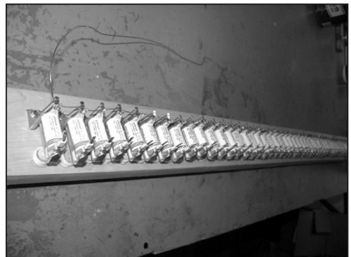
Figure 3. Another view of the manifold board from above—the copper wire on the left will be connected to the MIDI circuit board.
