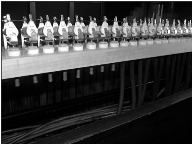
Figure 9. The rubber tubing is connected from the Tee to the cooper fitting on the bottom of the manifold board.
