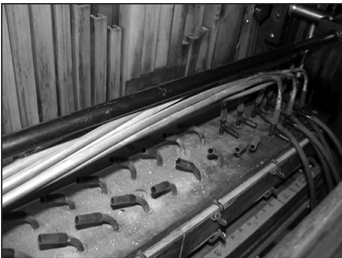
Figure 4. Bruder valve chest showing lead tubing cut to insert plastic Tees. Right-most Tees were inserted directly into the chest.
