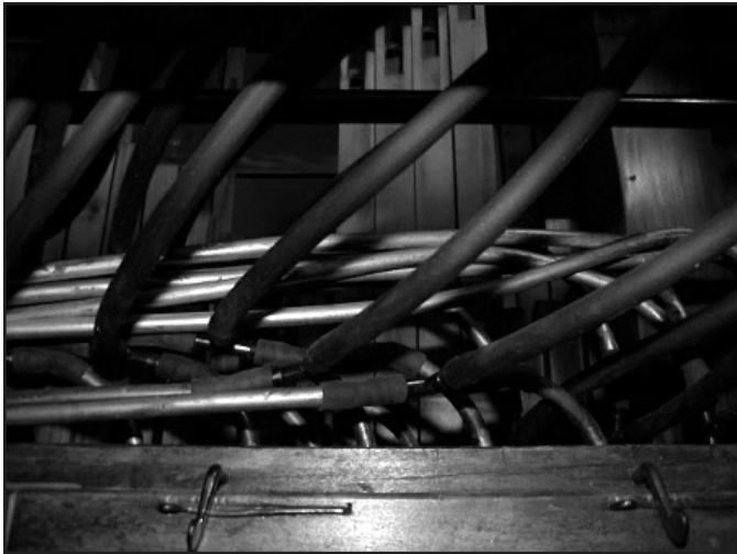
Figure 8. The ¼" rubber tubing is connected to the middle leg of the Tee.
